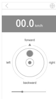
Move the button
