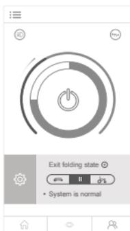
When H3S is powered off, click the contracting button and it will contract automatically. Click the extending button and it will automatically extend. Click the stop button, it will stop contracting or extending.
